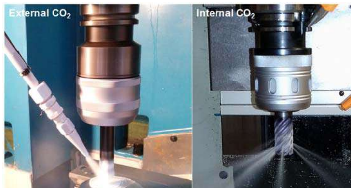
Fig. 1. CO 2 injected as external and internal coolant.
